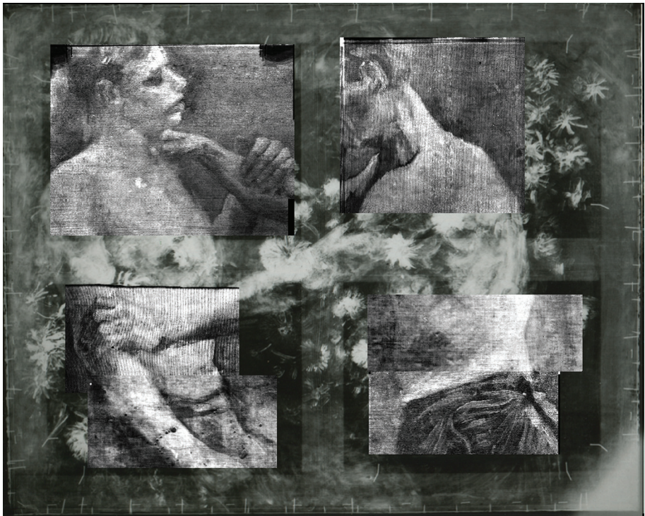
Four images showing the distribution of zinc white (ZnO), captured using MA-XRF from the verso at DESY (Hamburg) and the coarser scans at the Kröller-Müller Museum; overlaid with the X-ray image.
